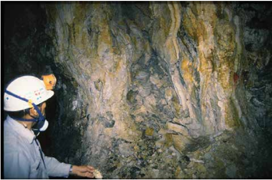
Typical gold-bearing quartz vein from an underground stope at Sumitomo's Hishikari gold mine in Japan. Photo courtesy Sumitomo Metal Mining Co. Ltd.
